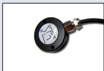
RFTO - Special probe for humidity/temp measurements in walls and boundary layers Operating conditions: -20...+80°C. D=30mm x H=10mm
