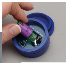
Changing the battery is very simple
